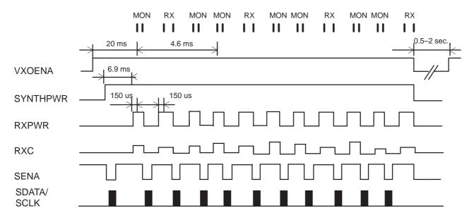
In case of long list of adjacent channels, there might be two monitoring– bursts/frame. Extra monitoring "replaces" TX–burst.
