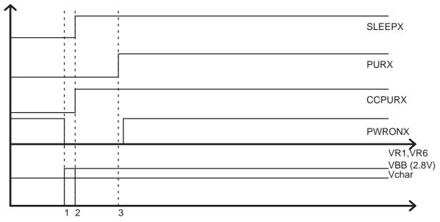
1:Power switch pressed ==> Digital voltages on in CCONT (VBB)
