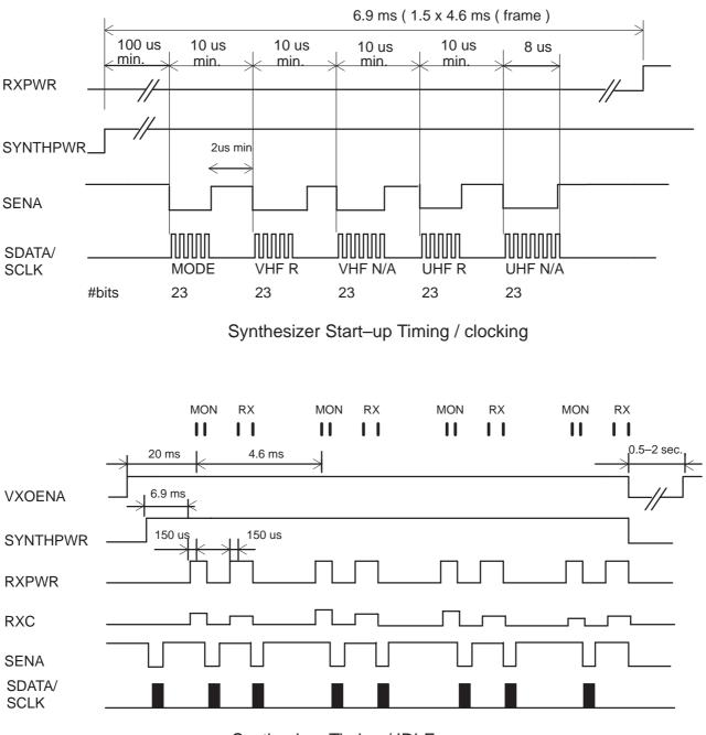
Synthesizer Timing / IDLE, one monitoring frame, frame can start also from RX–burst
